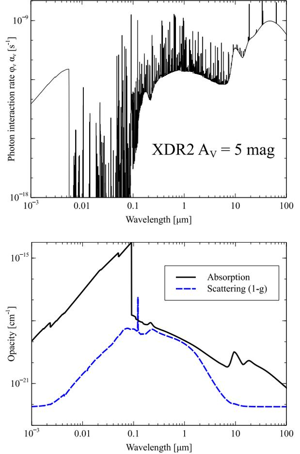
Fig. 7. Components of the radiation field at a depth corresponding to  $A_V = 5 \text{ mag}$  in the XDR2 simulation. The lower panel shows the absorption and scattering opacities while the upper panel shows the photon interaction rate.
