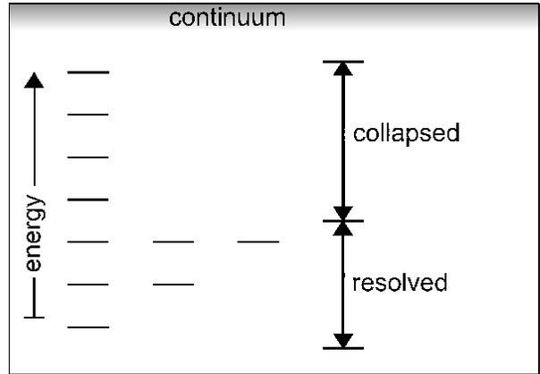
Fig. 1. The iso-sequence atomic level structure consists of low-lying  $nl$  resolved ( $nls$  for He-like) terms with  $l$ -mixed ( $ls$  for He-like) collapsed configurations. The number of resolved and collapsed levels can be specified when the simulation parameters are established.
