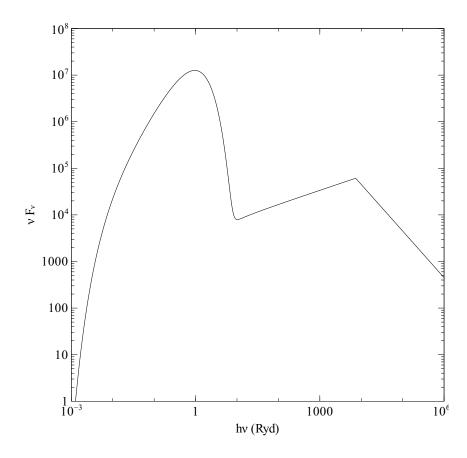
Figure 6.1: The continuum produced by the **AGN** continuum command. The Big Bump peaks at  $\approx 1$  Ryd, while the X-ray power law dominates at high energies. The two components are normalized by the second parameter, the value of  $\alpha_{ox}$ .
