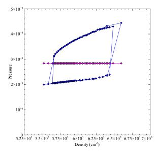
Figure 10.5: A thermal front in a constant pressure simulation. The x-axis gives the density [cm<sup>-3</sup>] and the y-axis is the pressure [dynes cm<sup>-2</sup>]. The points forming the large box are the resulting total gas pressure and the horizontal line is the correct pressure. The solution jumps above and below the equilibrium value as the temperature jumps above and below the thermal front.
