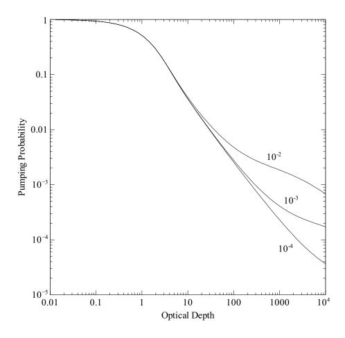
Figure 5.1: This figure shows the probability that a photon will penetrate to the line center optical depth shown on the x-axis, and then be absorbed by the line. The curves are for various values of the damping constant a (the ratio of damping width to Doppler width), as indicated on the figure.
