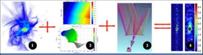
The end to end analysis, composed of a zoom-cosmological simulation coupled to an emission model processed by the instrument's model predicts that the CGM should be detectable by FIREBall-2's instrument.
