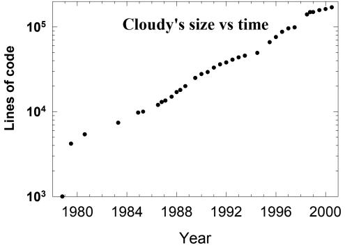
Figure 7 The size of the code, indicated by the number of lines of executable Fortran, as a function of time. size
