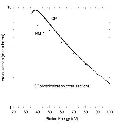
Figure 8 This figure shows the  $O^+$  photoionization cross sections now used, compared to the Reilman and Manson values, used in version 84 and before. o2photo
